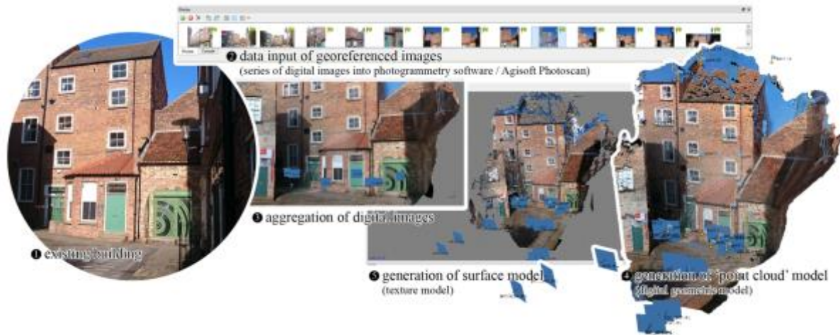
Fig. 5: Sequence of tasks for undertaking ground level photogrammetry survey.
