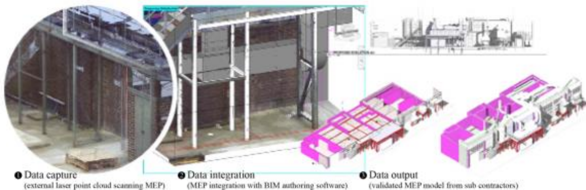
Fig. 10: LiDAR ground level survey of complex services.
